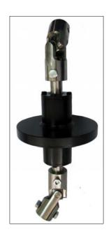
Designed to provide a fixed point of rotation and support the weight of rigid rod, our Intermediate Coupling comes equipped with shaft collar and thrust bearings to provide smooth transmission of torque.
